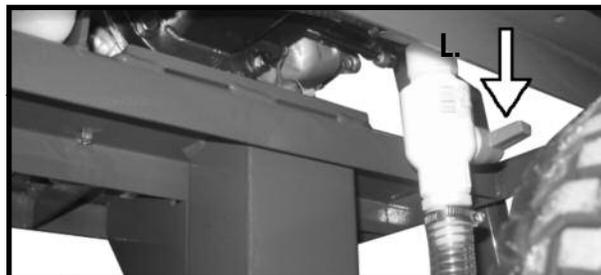
5. To drain tank, rotate the drain valve (L.) 90° allowing flow from the drain hose. To completely drain tank, remove the lower housing of the in-line filter (M). \*After draining, clean the filter, replace the housing and close the drain valve (L) ensure that upon refilling the tank chemical will not drain out of the un
