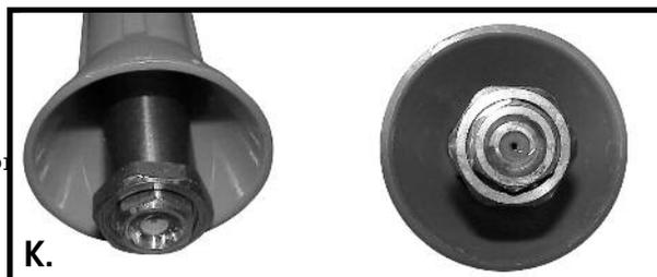
3. Replace the spray gun tip every season. As the hole in the tip gets larger the spray pressure drops and degrades the quality of the spray. (K)
