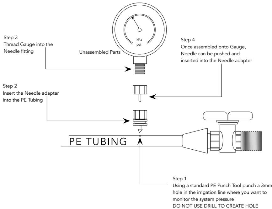
A single Gauge/Needle can be used for multiple locations that have Needle adapters. Removing the Needle from the Needle adapter, the internal bladder reseals and no leak is created.
